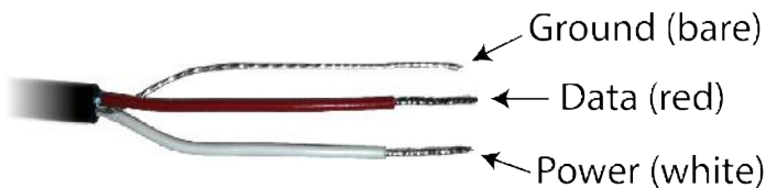
Figure 6: Pigtail End Wiring
